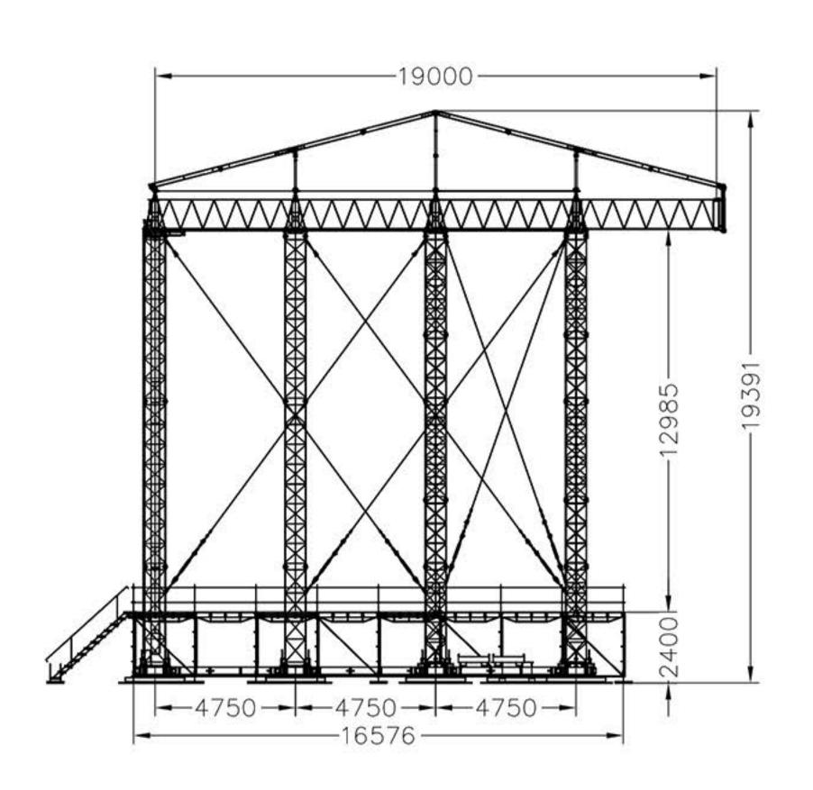
The AES 4-Leg Classic is a versatile roof, designed for all types of outdoor staging. This stage has a proven track record in the Middle East over the past 15 years, being the stage of choice for the world's best artists.
